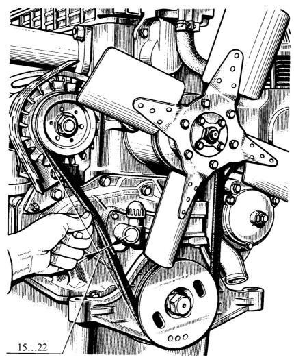
Fig. 14 – Checking the fan belt tension.
