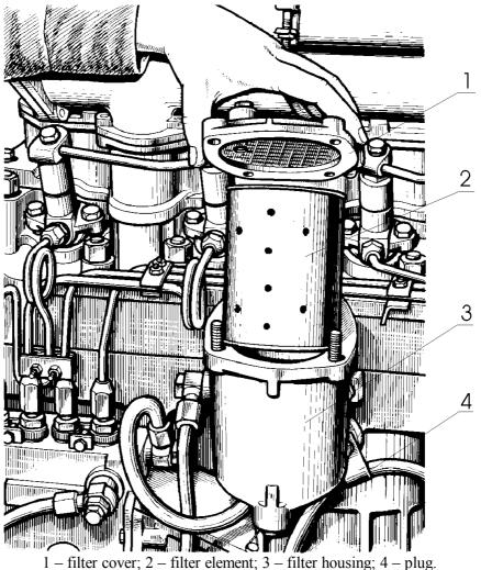
Fig. 22 - Replacement of the filter element of the fine fuel filter.
