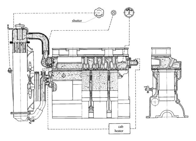
Fig. 10 – Diagram of the Cooling System
