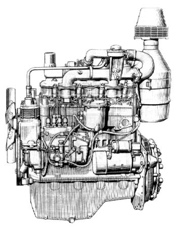
Fig. 5 – D-245 Diesel Engine (Left View).
