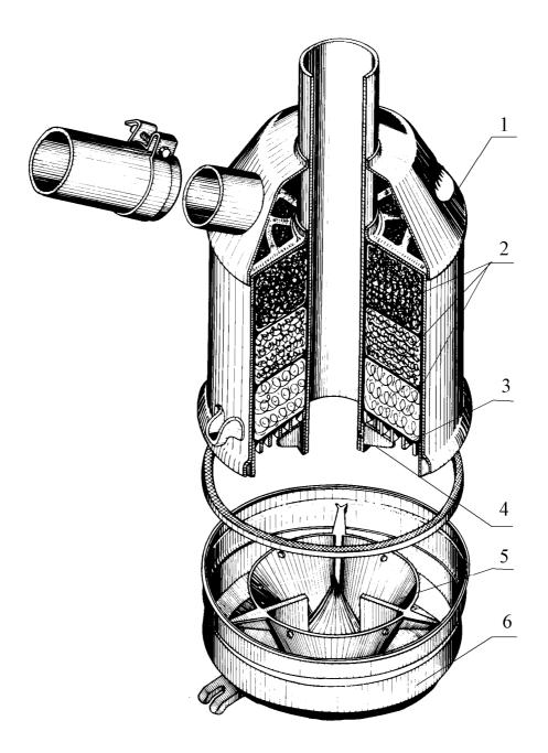
1 – air-cleaner housing; 2 – filtering elements; 3 – holder; 4 – holder stopper; 5 – oil reservoir; 6 – pan.
