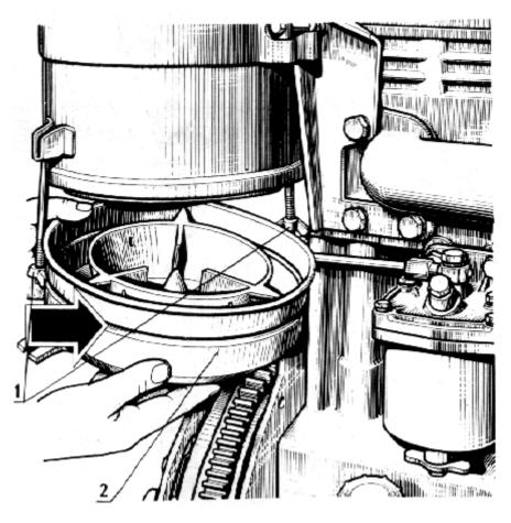
1 - nut; 2 - pan.Fig. 15 – Checking the oil level in the air cleaner pan.
