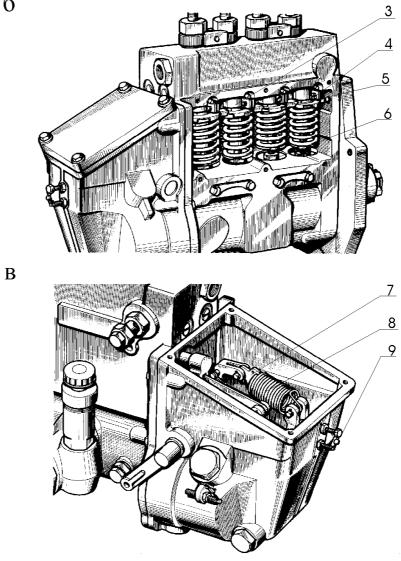
1 - adjusting screw; 2 - nominal bolt (stop); 3 - teeth crown; 4 - fixing screw; 5 - rotating bush; 6 - pusher adjustment bolt with lock nut; 7 - shackle; 8 - governor spring; 9 - idling spring adjustment bolt.
