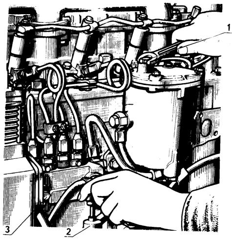
1– fitting; 2 – priming pump; 3 – plug. Fig. 23 – Removal of air from the fuel system.
