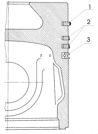
1 – upper compression ring; 2 – conic compression ring; 3 – oil ring. Fig. 33 – Diagram of mounting the piston rings.
