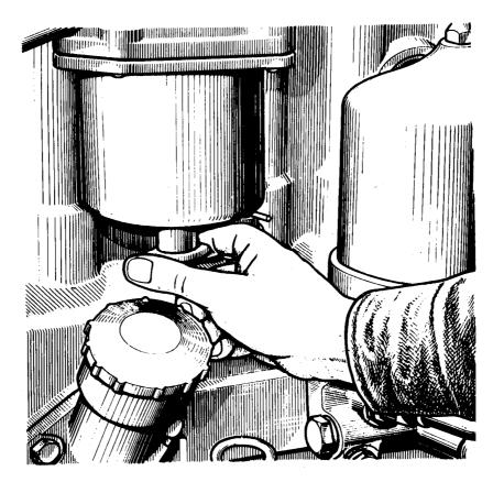
Fig. 13 – Draining the coarse fuel filter.
