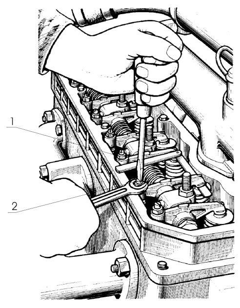
1 – lock nut; 2 – screw.Fig. 18 – Adjusting the clearance in the valves.
