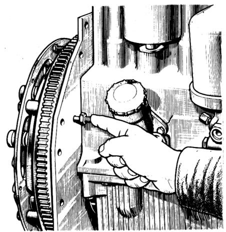
Fig. 27 – Setting the splint into the hole of the rear sheet and flywheel.
