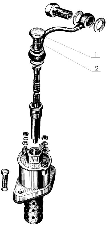
1 – pipe connector bolt; 2 – hole Fig. 32 – Electric torch pre-heater.
