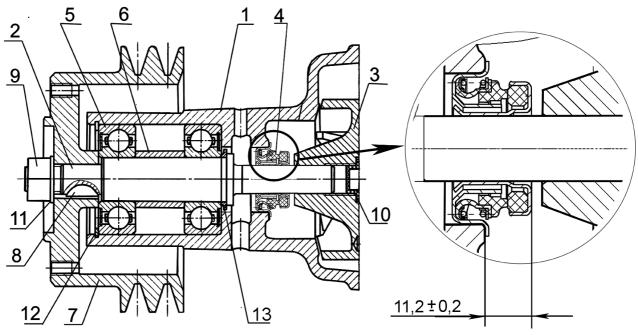
1 – Case; 2 – pump shaft; 3 – impeller; 4 – water pump sealing SP/1341; 5 – bearing; 6 – sleeve; 7 – sheave; 8 – dowel; 9 – nut; 10 – cap screw; 11 – washer; 12 – stop ring; 13 – sealing ring. Figure 35 – Water pump
