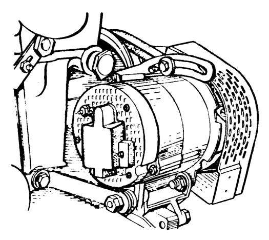
1 – seasonal voltage adjustment screwFig. 31 – Seasonal adjustment of the alternator voltage
