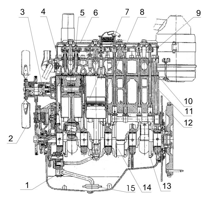
1 – oil pump; 2 – fan; 3 – water pump; 4 – piston pin; 5 – connecting rod; 6 – cap; 7 – piston; 8 – cylinder sleeve; 9 – cylinder head cover; 10 – cylinder head; 11 – cylinder block; 12 – flywheel; 13 – counterweight; 14 – crankshaft; 15 – oil collector.
