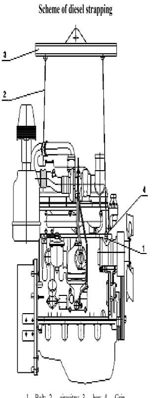
1 - Bolt; 2 - circuitry; 3 - bar; 4 - Grip Figure 36 - scheme of diesel strapping
