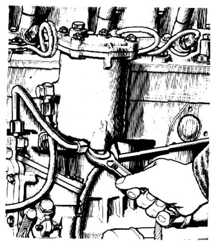
Fig. 19 – Draining the fine fuel filter.
