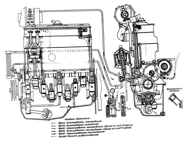
1 - oil radiator; 2 - piston cooling fuel injectors; 3 - centrifugal oil filter; 4 - protective strainer; 5 - oil-filler neck; 6 - plug of the oil sump; 7 - reducing valve; 8 - drain valve; 9 - pressure gauge; 10 - safety valve; 11 - oil receiver; 12 - oil pump.
