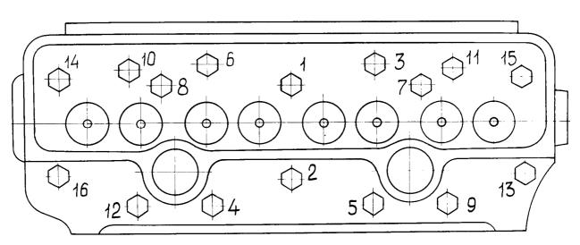
Fig. 21 – Diagram of the order of tightening the bolts fastening the cylinder head.
