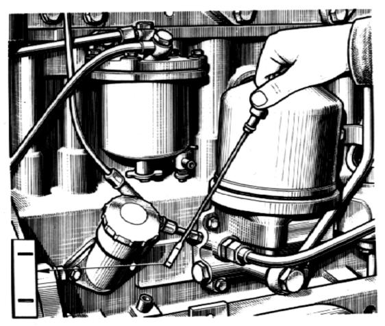
Fig. 12 – Checking the oil level in the diesel engine crankcase.
