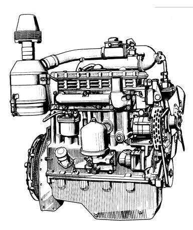
Fig. 2 – D-243 Diesel Engine (Right View)
