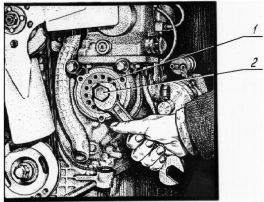
1 – slotted flange of the pump gear; 2 – fuel pump shaft nut. Fig. 29 – Adjusting the diesel engine timing
