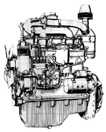
Fig. 1 – D-243 Diesel Engine (Left View).
