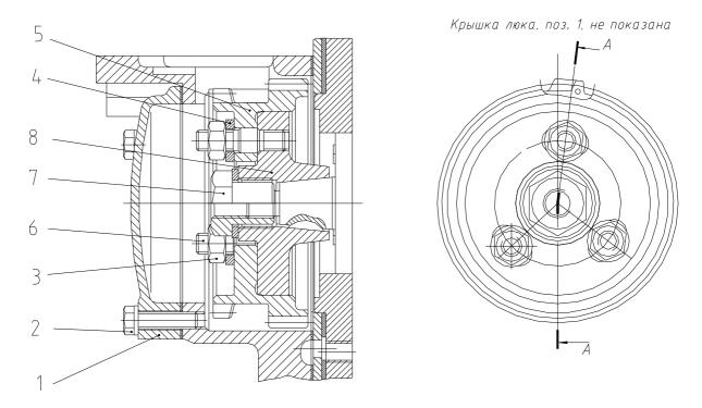
1 – adjusting bolt; 2 – bolt; 3 – nut; 4 –washer; 5 – fuel pump drive gear; 6 – stud; 7 – nut, special, 8 - flage
