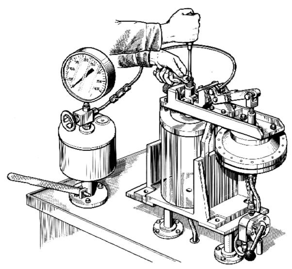
1 - adjusting screw; 2 - lock nut.Fig. 30 - Adjusting the fuel injector.
