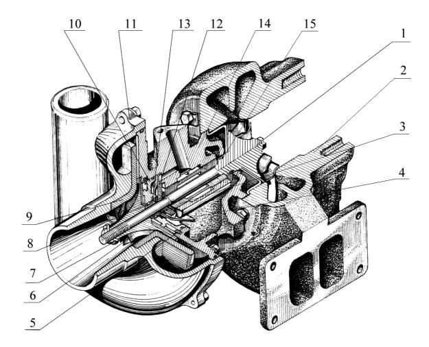
1 – turbine wheel with shaft; 2 – turbine housing; 3 – mono-bush; 4 – oil-guard; 5 – eccentric ring; 6 – compressor wheel; 7 – special nut; 8, 15 – O-rings; 9 – diffuser; 10 – cover; 11 – compressor housing; 12 – thrust bearing; 13 – distance bush; 14 – middle housing (housing of bearings). Fig. 9 – Turbo-supercharger.
