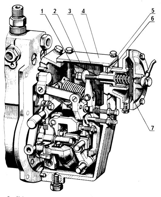
1 – lock nut; 2 – stop; 3 – rod; 4 – cover; 5 – dowel; 6 – bush; 7 – diaphragm. Fig. 26 – Adjusting the fuel pump with antismoke corrector.
